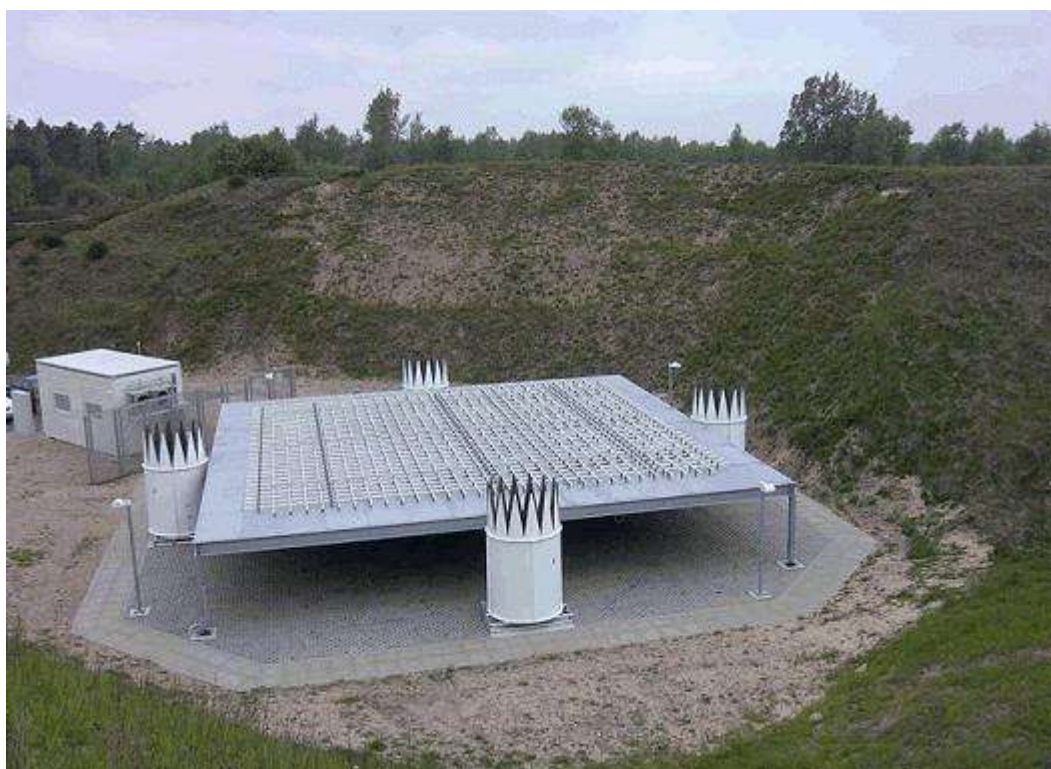
Fig.4.9 A schematic representation of a Wind Profiler
