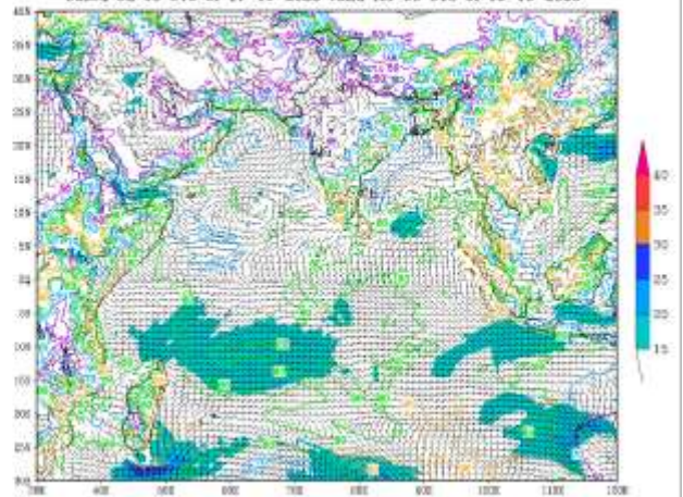
IMD GFS (T1534) 10m WIND (kt) AND 2m RH (%) FORECAST (48 HR) based on 00 UTC of 17-10-2023 valid for 00 UTC of 19-10-2023
