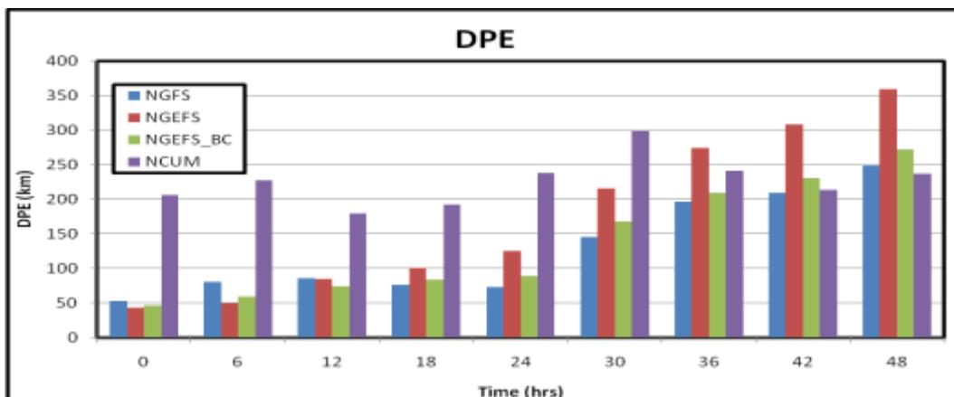
Fig.13 Direct position errors (DPE) for NGFS, NGEFS, NGEFS\_BC and NCUM models based on 6-8<sup>th</sup> November 2014 initial conditions
