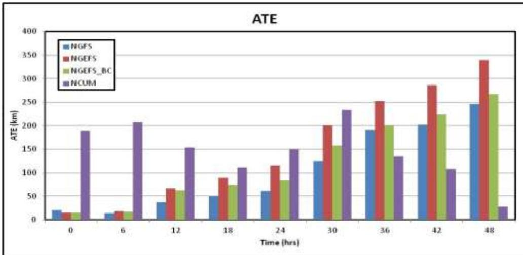
Fig.11 Along track errors (ATE) for NGFS, NGEFS, NGEFS\_BC and NCUM models based on 6-8<sup>th</sup> November 2014 initial conditions
