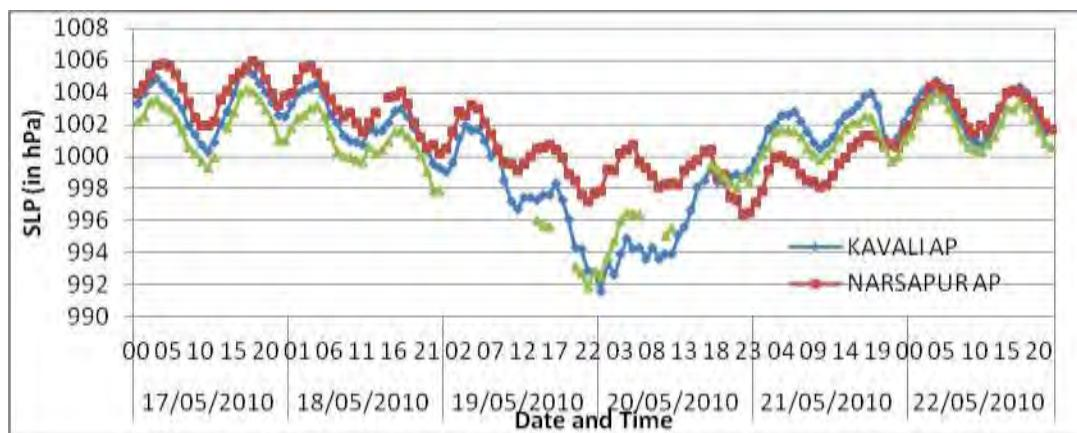
**Fig. 2.7: Variation of sea level pressure (SLP) recorded at AWS as the cyclone —AILA— approached the coast.**
