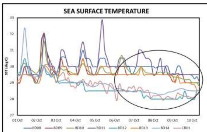
**Fig. 2.2.6 Sea Surface Temperature recorded by the buoys during 1-10 October**
